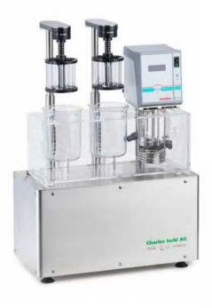
The **DISI-A**, seen here with two measurement stations, is operated via the PH21 computer software
